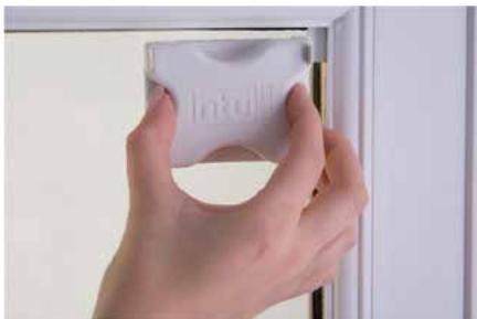
4. Insert the bracket behind the rubber seal until the tool edge touches the bead at both top & side. Repeat for other side.
