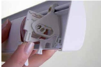
11. Check the position of the 'blind to fascia' retaining brackets are as shown. If not press the finger release lever and move to open position as pictured. Repeat at opposite end. As blind is pre-tensioned do not remove blind from fascia brackets.
