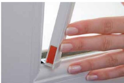
7. Side profiles should be evenly vertical. If the window is not square, attach pads supplied on side of profile as needed. Locate the profile bottom end cap over the bottom bracket.
