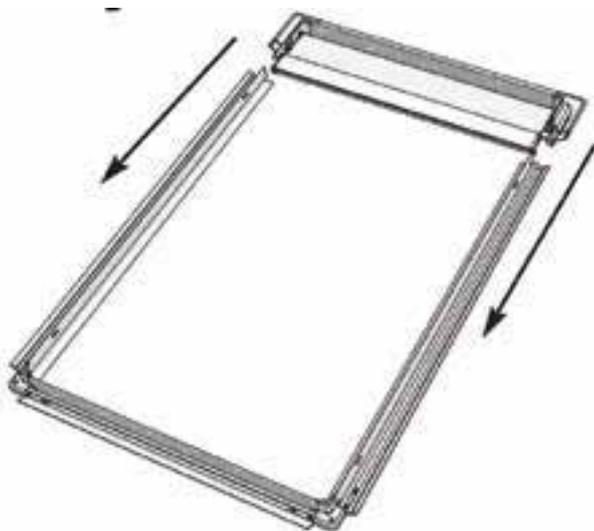
Slide the top section into the rest of the frame, attach the end caps and then tighten the screws on each joint.
